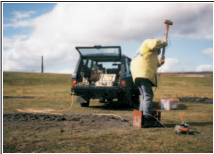
Down-hole Shear wave survey through colliery spoil, South Wales
